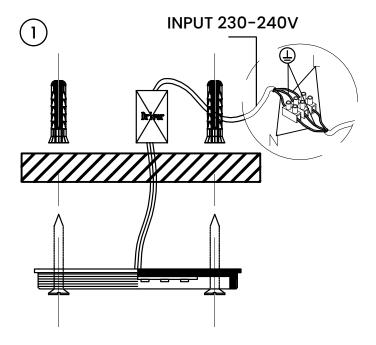
Connect the main power to "L" and "N" terminal block. Fix the ceiling pan.
