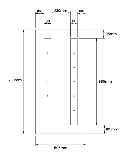
FINISH: **MATERIAL**: Acoustic Felt, Timber LIGHT GREY Thickness: 25mm GREY DARK GREY
